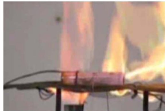
After the electrolyte has gushed out, it catches fire in the burner flames and burns violently. (The above photograph was taken with a normal camera).
