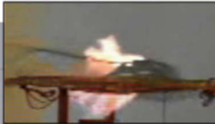
- When the area around the battery is heated to 240 °C - The battery bursts into flames with a loud noise.
