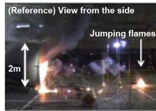
Test conducted inside a steel tank for safety purposes Flames jumped out of the tank
