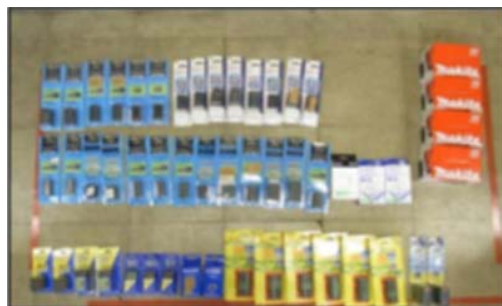
The lithium ion batteries used in the test 95 lithium ion battery packs (480 cylindrical cell batteries of 18 mm diameter and 65 mm length) of the type used in video cameras and so on
