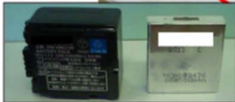
Commercially available lithium ion battery (left side): 2 single cells are contained.
