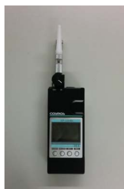
Figure 13 Odor sensor used for confirming leakage
